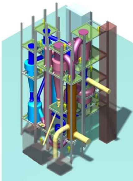
**Figure 5. Layout of the Taylor Gasification Process**
