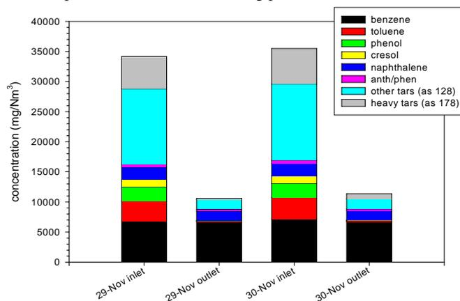
**Figure 4. Consistent Performance of the Gas Conditioning Step**
