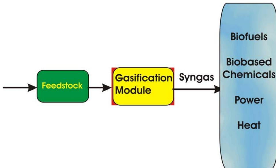
The Taylor gasification process, being developed by Taylor Biomass Energy is a biomass gasification process that produces a MCV gas. MCV gas, unlike the low calorific value gas produced in air blown gasifiers, provides the ability to achieve the goal of a true biomass refinery capable of producing not only a fuel gas or power but a range of products.
